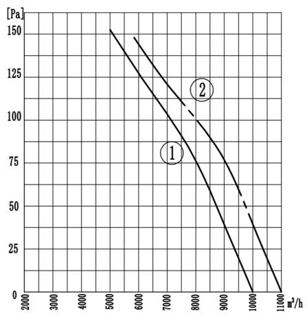
Curve 1: 50HZ Curve 2: 60HZ
